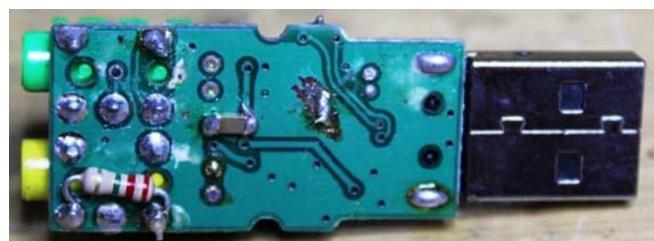
'3D Sound' soundcard with soft-clip circuit modifications as shown in schematic below.
