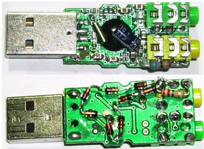
MIC socket input is mono, with phantom MIC powering via 4.5VDC to socket from chip bias supply, and then 100nF coupling cap to CM108 MICIN pin. Modifications made:
