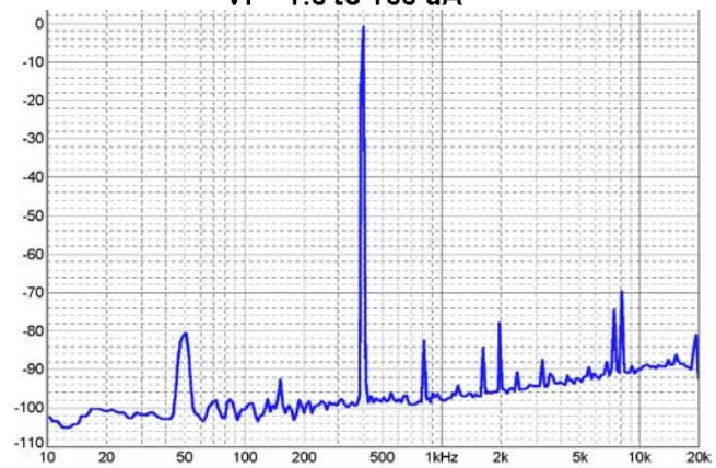
The results below are for 2Vrms and 3Vrms levels from a TMC oscillator. The 3Vrms input level shows substantial soft clipping above an ADC input voltage of about 0.7Vpk (the scale is about 0.35Vpk/div), which indicates diode current may only be peaking near 1uA. Although there are exotic (and expensive!) diodes
