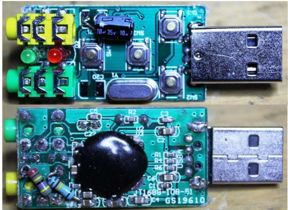
'7.1 Channel Sound' virtual soundcard with just the basic modifications shown in schematic below (no protection clipper parts). The circuitry appears to be fairly similar to the '3D Sound' device, and is modified in the same manner.
