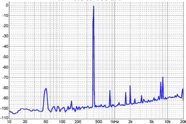
The results below are for 2Vrms and 3Vrms levels from a TMC oscillator. The 3Vrms input level shows substantial soft clipping above an ADC input voltage of about 0.7Vpk (the scale is about 0.35Vpk/div), which indicates diode current may only be peaking near 1uA. Although there are exotic (and expensive!) diodes
