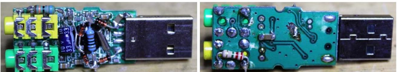
'3D Sound' soundcard with soft-clip circuit modifications as shown in schematic below.
